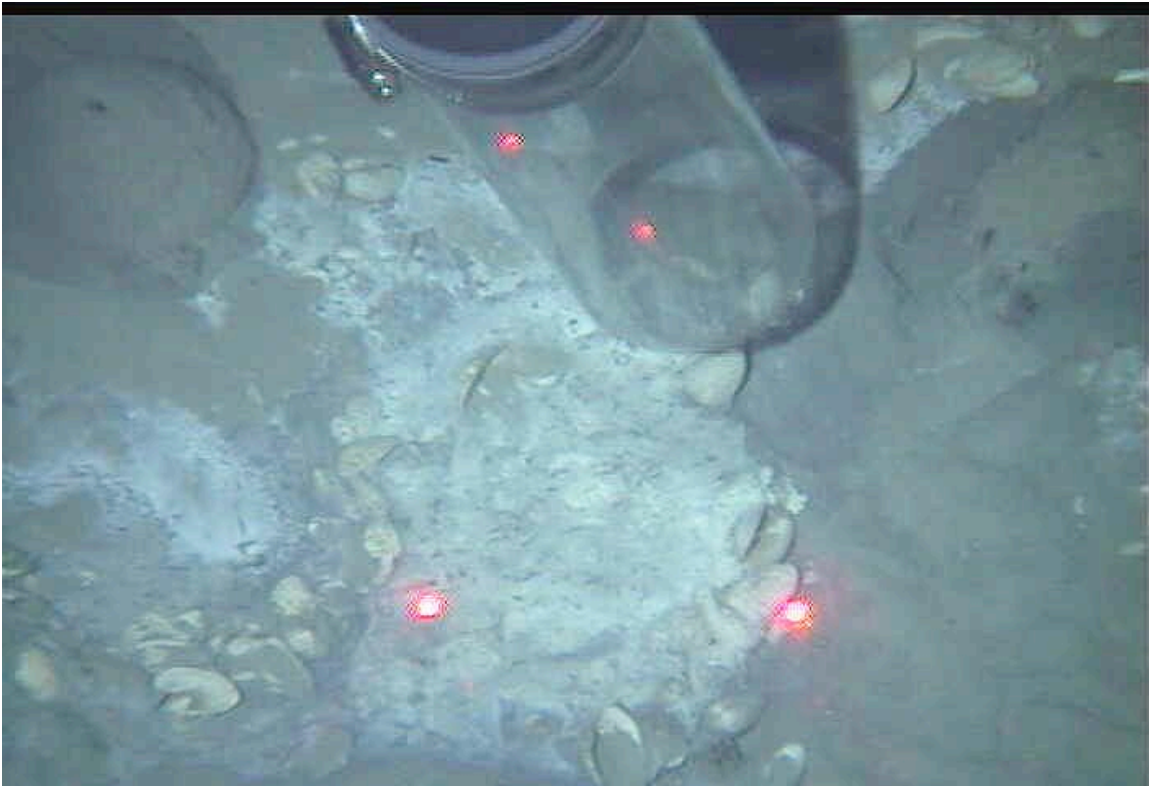
Push core sampling of a thick, white bacterial mat associated with live clams. The red laser dots are 10 cm apart.
