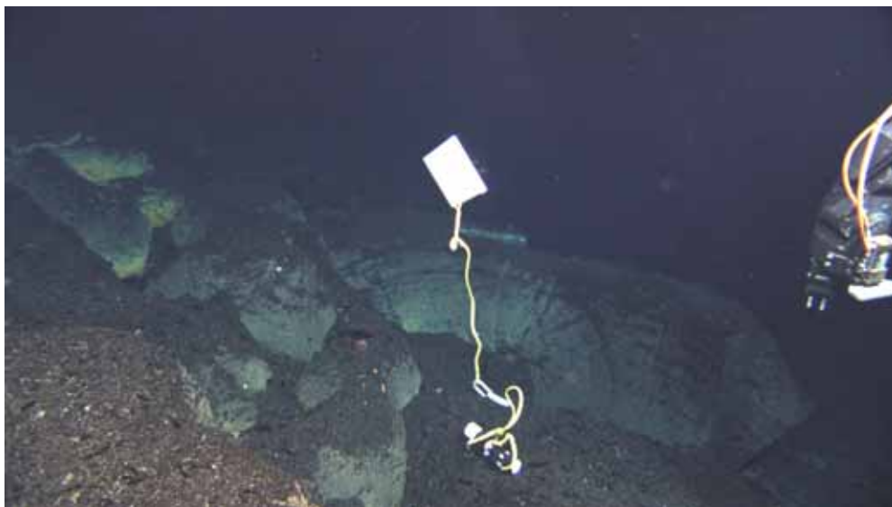
B-Probe hydrophone deployed at Mkr-147, dive J2-413
