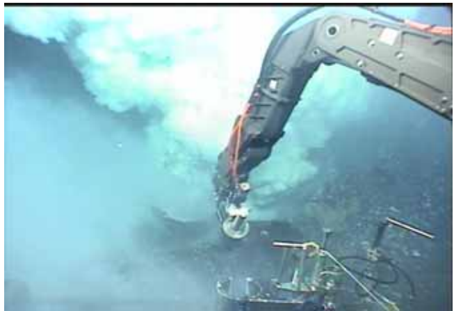
(left) Dive 413 Major at Prometheus 1175m depth before sampling. (right) Dive 413 Major (sample 10) at Prometheus just after triggering. 2009/05/06 20:21:57. Sampler obscured by smoke during triggering. Large amount of seawater in this sample. Only other samples this dive were two Niskins in the plume at the end of the dive. NO TEMPERATURE MEASUREMENT.
