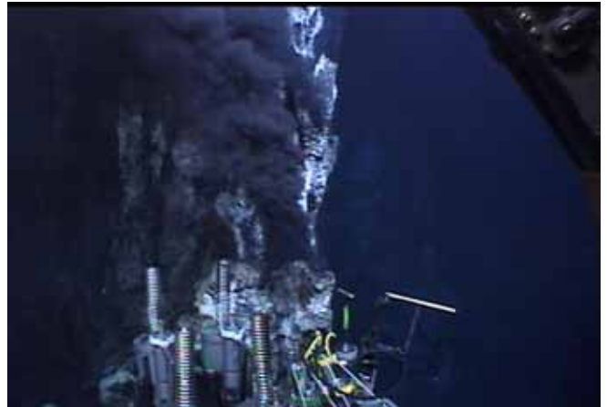
(left) Dive 416 2009/05/09 14:25:07 Taking black major in 315°C orifice. depth 1525, heading 140. (right) Dive 416 16:22 View of 315°C black smoker where all majors were taken at Maka volcano.
