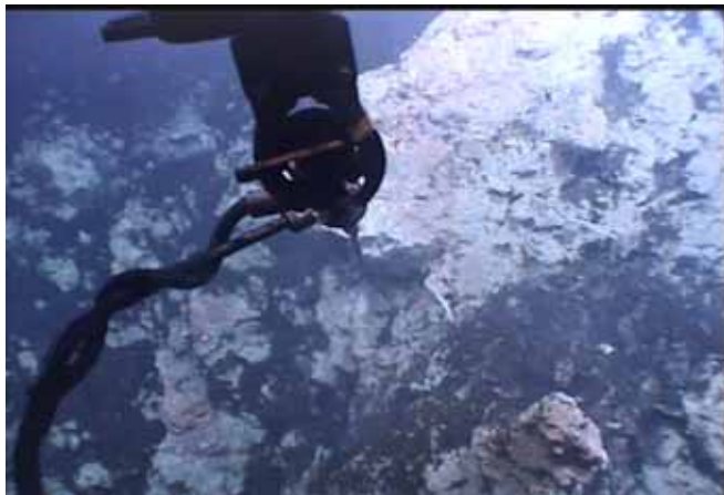
(left) Dive 417 2009/05/10 10:20:24 Measured average pH of 4.22 at 17.4°C, H 2 S voltage 0.281 at start of sampling, but the manifold was not flushing well. Later at this same site, got good flow, with pH of 2.599, H 2 S voltage 0.393, and average 28.0°C. (right) Dive 417 2009/05/10 10:31:13 Down-looking view of HFS setup at Epsilon site, near Red Rock Ridge. Collected bag 22, 23 (failed), 19, sterivex 14. No gas-tight here.
