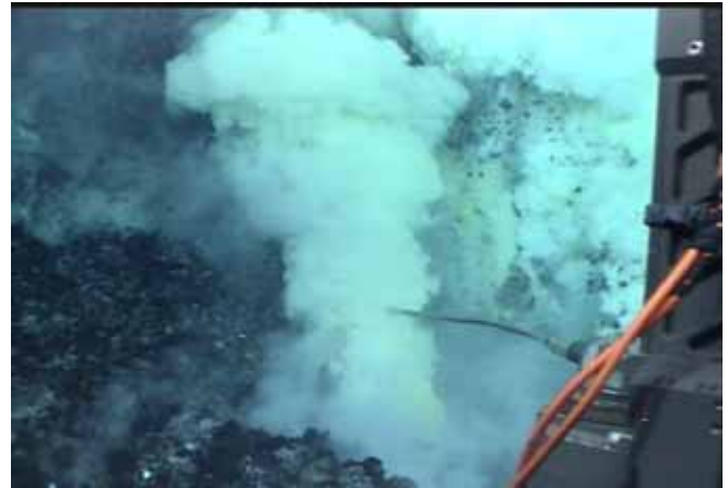
(left) Dive 418 2009/05/11 14:42 Conditions at start of filtered piston #5 at Afi vent. (right) Dive 418 14:43:47 Still taking HFS filtered piston 5 at Afi. Note tephra produced at vent to the right.
