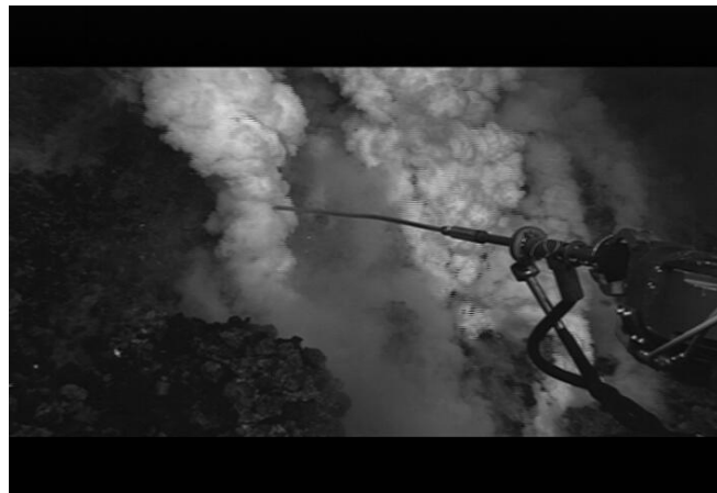
(left) Dive 418 2009/05/11 14:30 View of "Akel's Afi" (Z=1198 heading 220). This vent was flaming and producing some tephra. The flame would periodically light and extinguish itself. (right) Dive 418 14:37 Setting up to sample the jet on the left. The vent on the right is producing lots of tephra and flaming. The tephra would clog the sampler, so will try the one on the left.
