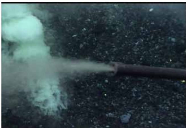
(left) Dive 418 2009/05/11 12:58 Reverse flow on HFS blowing out fine particles from the manifold. (right) Dive 418 13:20 Taking green discrete gas-tight at Hades, very close to the point of the fluid sample inlet for previous HFS samples here.
