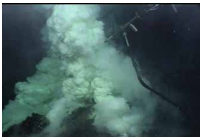
(left) Dive 414 2009/05/07 13:10:03 HFS setup at Prometheus vent. Many of the samples taken here failed due to probable clogging. (right) Dive 414, 2009/05/07 13:29:41 Sampling unfiltered piston 6 in plume over Prometheus. Also fired starboard HFS gas-tight at this time.
