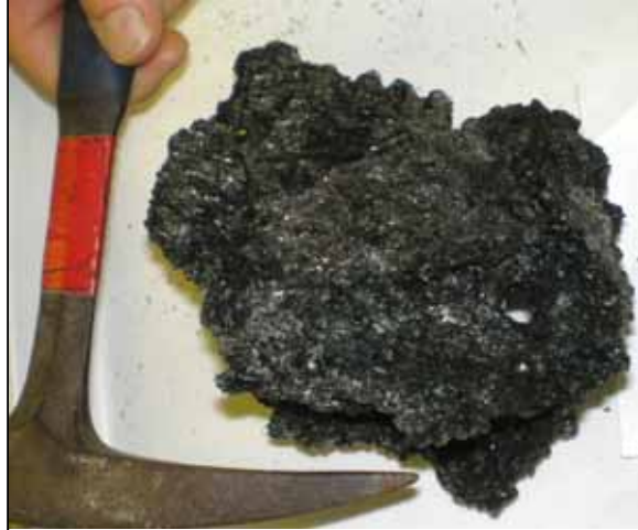
Sample J2-420-R23 as it appeared on deck. The hole left by the sampling rod is visible at the right.
