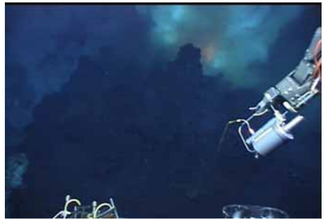
(left) Dive 420 2009/05/12 21:22 (Z=1196 heading 16). Sampling grayish fluids emanating from actively forming pillow lava mound. Dive sample number 20, Black major #11C. (right) Dive 420 21:29 (Z=1194 heading 168). Flaming vent in background, preparing to take yellow major just below the view in this frame.
