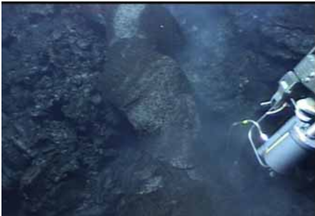
(left) Dive 420 21:31 Taking yellow major #6C in cloudy fluid emanating from recently formed pillow mound. This is 4 meters below the flaming volcanic vent. (right) Dive 420 21:36 Firing red gas-tight in same spot where two major samples were taken.
