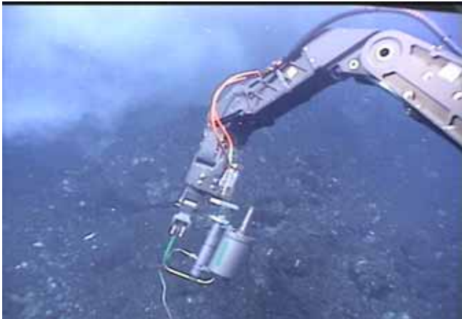
(left) Dive 413 Major at Prometheus 1175m depth before sampling. (right) Dive 413 Major (sample 10) at Prometheus just after triggering. 2009/05/06 20:21:57. Sampler obscured by smoke during triggering. Large amount of seawater in this sample. Only other samples this dive were two Niskins in the plume at the end of the dive. NO TEMPERATURE MEASUREMENT.
