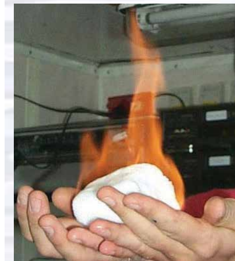
Methane hydrate looks like ice, but as the "ice" melts it releases methane gas which can be a fuel source. Image credit: Gary Klinkhammer, OSU-COAS
