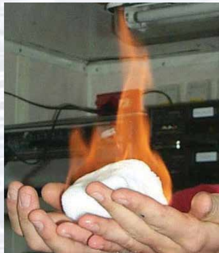
Methane hydrate looks like ice, but as the “ice” melts it releases methane gas which can be a fuel source. Image credit: Gary Klinkhammer, OSU-COAS
